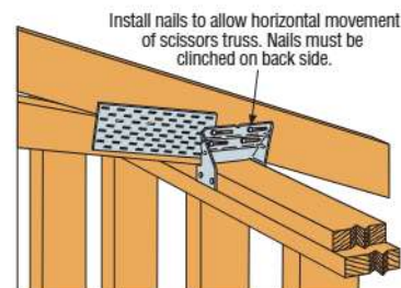
Typical TC24 Installation
